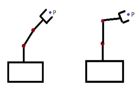
1. Revolute joint is measured by an angle moving counterclockwise. Denoted as S and its parameter is from zero to  $2\pi$
